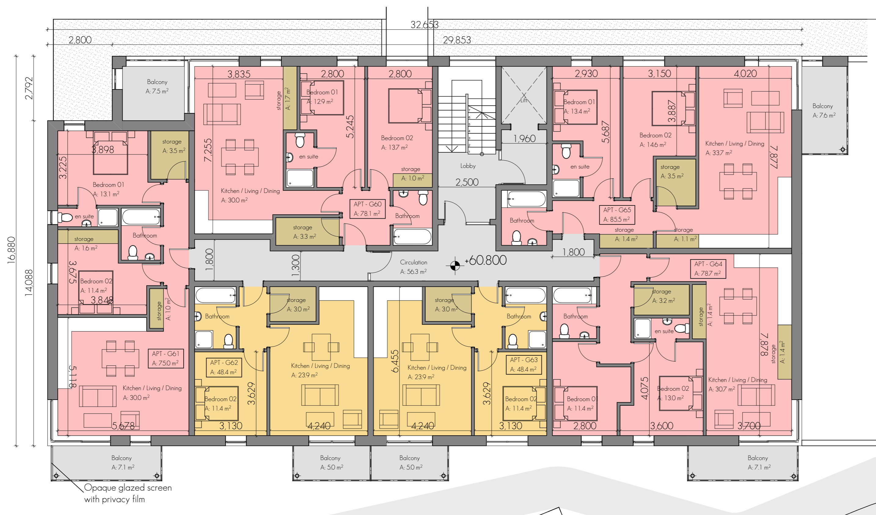
FIRST FLOOR PLAN - BLOCK B THIS IS THE TYPICAL UPPER FLOOR PLAN FOR THE 1ST, 2ND & 3RD FLOOR - FLOOR LEVEL- 1ST_60.800 - 2ND_63.725 - 3RD_66.650 1:100
